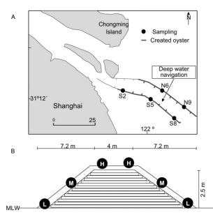
Figure 1. (A, B) Location of the created intertidal oyster reef in the Yangtze River estuary (A) and a schematic drawing of the sampling transect and cross-section of the artificial reef (B). High (H), middle (M), and low (L) intertidal zone, as well as mean low water (MLW) during spring tide are labeled.
